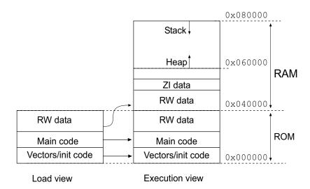
Figure 6-5 Memory map for simple scatter-loading
