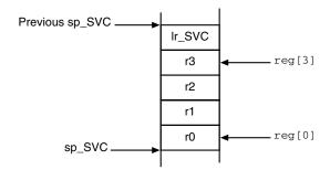
Figure 5-2 Accessing the supervisor stack
