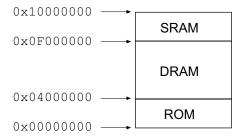
Figure 6-1 Example of a system with ROM at 0x0
