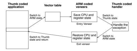
Figure 5-4 Handling an exception in Thumb state
