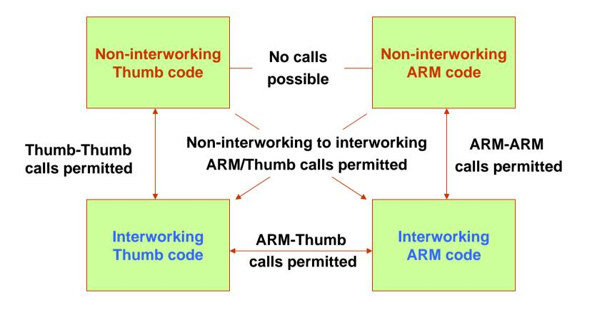
Modules that are compiled for interworking generate slightly larger code, typically 2% larger for Thumb and less than 1% larger for ARM.
