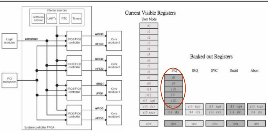
The ARM fast interrupt (FIQ) architecture includes more banked registers than the other exception modes in order to minimize the register save and restore overhead associated with handling one of these interrupts.
