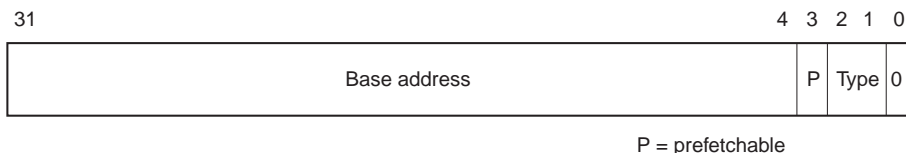
Figure 9-6 Base address for PCI Memory space
