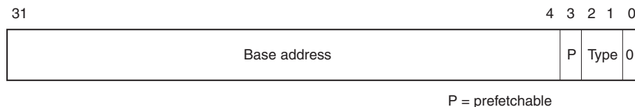
Figure 8-6 Base address for PCI Memory space
