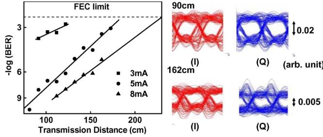
Fig. 5.  $-\log(\text{Bit Error Rate})$  versus transmission distance under different photocurrents during 1.25 billion symbols per second QPSK data transmission. Measured  $I$  and  $Q$  eye patterns under an 8-mA photocurrent at 90 and 162 cm are also specified.
