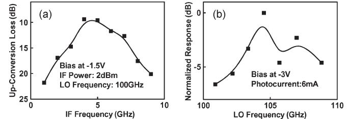
Fig. 3. (a) Frequency response of the up-conversion loss of our QPSK data transmission system measured under a fixed LO frequency (100 GHz) and different IF frequencies. (b) Measured O-E frequency response under different LO frequencies without IF injection.
