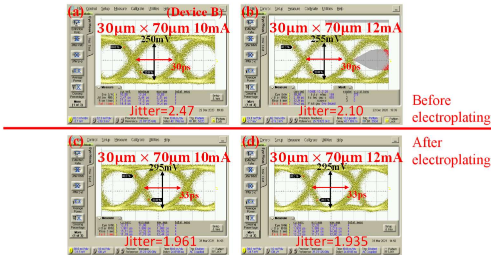
Figure 13. Measured 25 Gbit/sec eye patterns of device B under 10 and 12 mA bias currents and with a 30 \times 70 \mu\text{m}^2 active mesa size before (a) - (b) and after (c) - (d) the electroplating process.
